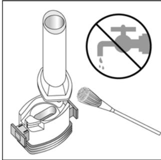
9. After you have used up all the powder, open the capsule chamber (see step 2). Remove the empty capsule and use a dry tissue or a soft brush to remove any powder left inside. Note: DO NOT USE WATER to clean the Aerolizer.
